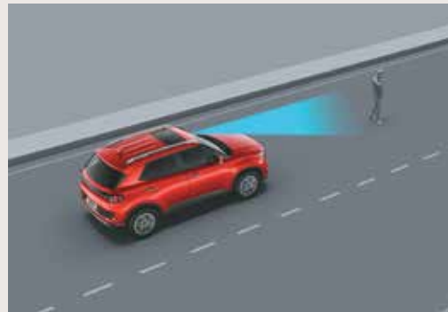
Forward Collision - Avoidance Assist - Pedestrian (FCA-Ped)
