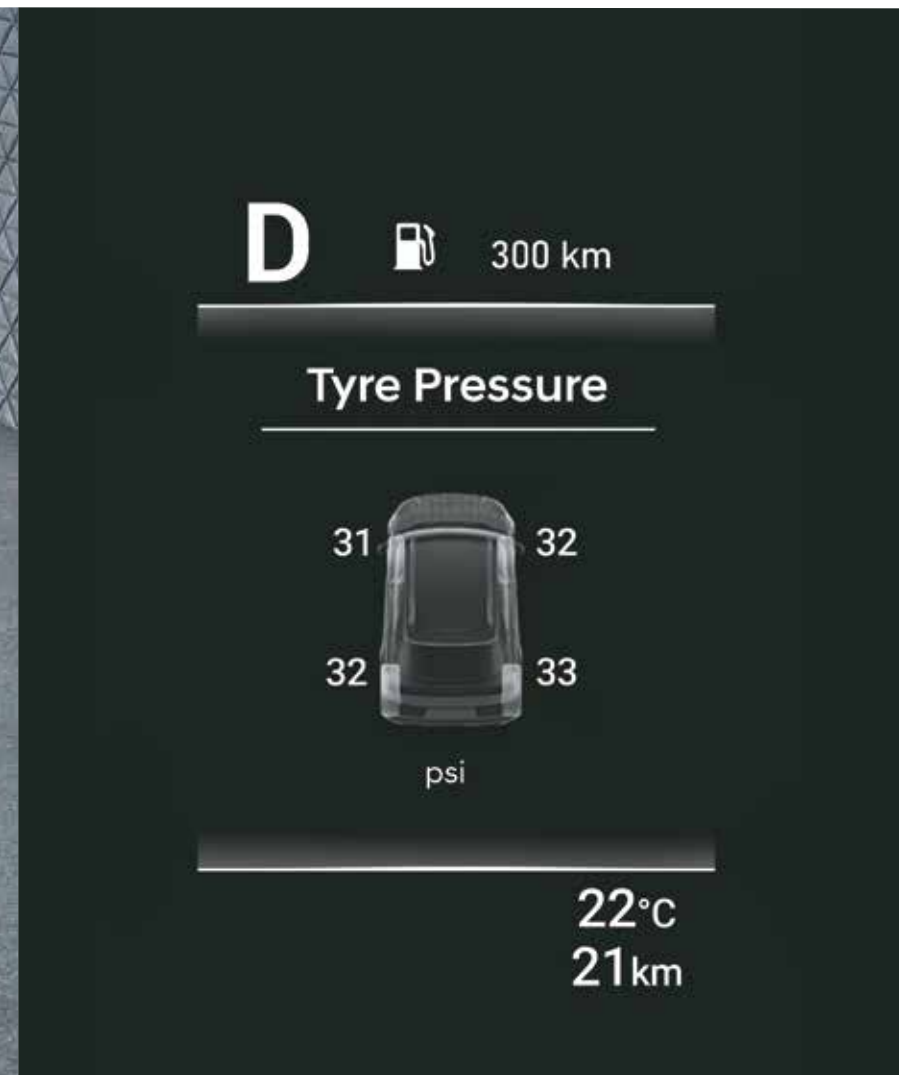
Tyre pressure monitoring system (Highline)
